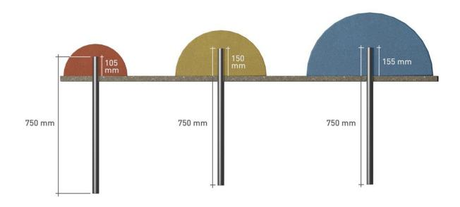
Outside - diameter metal pipe approx 42mm Inside - diameter pipe approx 38mm
