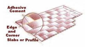
**Required quantity of glue**: 1 cartridge (310 ml) for every 3 – 4 m of joint length glued.
