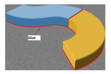
2. The EUROFLEX® C & S Blocks can also be used without being glued to the Underground, can be used directly in a fresh concrete bed (B15 dimensionally stable). For this purpose, several galvanized hexagon screws 10 x 200 mm, at least 70 mm deep, are screwed into the rubber and inserted with the screw head into the fresh concrete. Glue or joint the joints of the block steps together.
