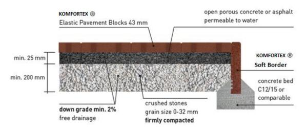
Note: The basement is taken off till attended depth plus thickness of the blocks. Through acceptance inspection for the subgrade is recommended for installation the blocks.
