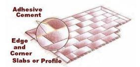
Required quantity of glue: 1 cartridge (310 ml) for every 3-4 m of joint length glued. Type of glue: elastic 1-component polyurethane adhesive cement Ottocoll P 83 grey and Ottocoll M 500 red available through us.
