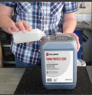
Open both components and pour component B (hardener) completly into the canister.
