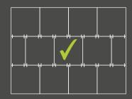
To fix the tiles to the wooden slats, screws are screwed at a distance of approx. 3cm from the corner of the tile and in such a way that the screw screws into the wooden slat, the screw head disappears into the tile and the tile is pressed against the wooden slat. In addition, a screw is used in the middle of the panel. For a 1,000 mm wide panel, eight screws are to be used.
