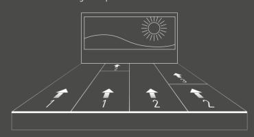
SPORTEC® rolls should be laid with pressure on the butted joints (close to overlapping). No welding or joint filler is required.
